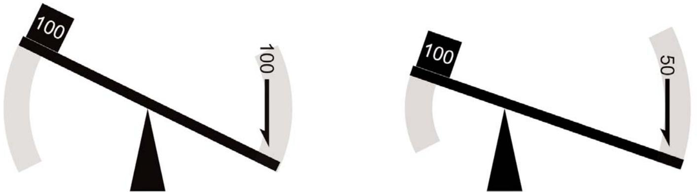
If the lever arm that the force is pushing down is twice as long as the arm with the weight, half the force is required to lift it. In this example 50 lbs. of force could lift 100 lbs. of weight but the force would travel twice the distance of the weight to do so.
