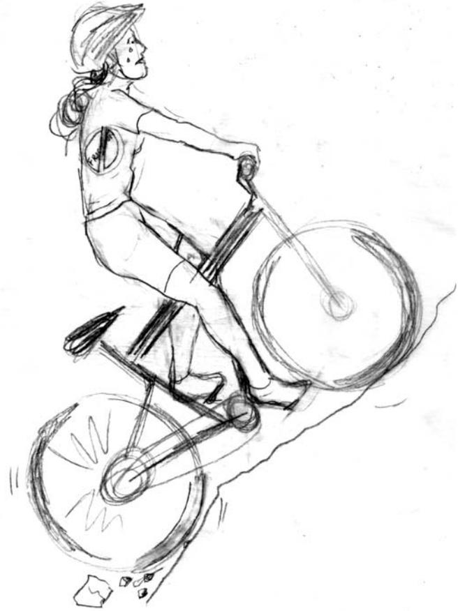
When the bike encounters inclined, slippery, or loose surfaces it is critical that the weight be over the drive wheel. If too much of the weight on a bike is over the front wheel, **gravity** will fail to hold the rear wheel down and traction (**friction**) will be lost. Whatever the design of your vehicle is be sure the weight is over the drive wheels. Traction is the reason most cars have their engine (the heaviest part) over the drive wheels.
