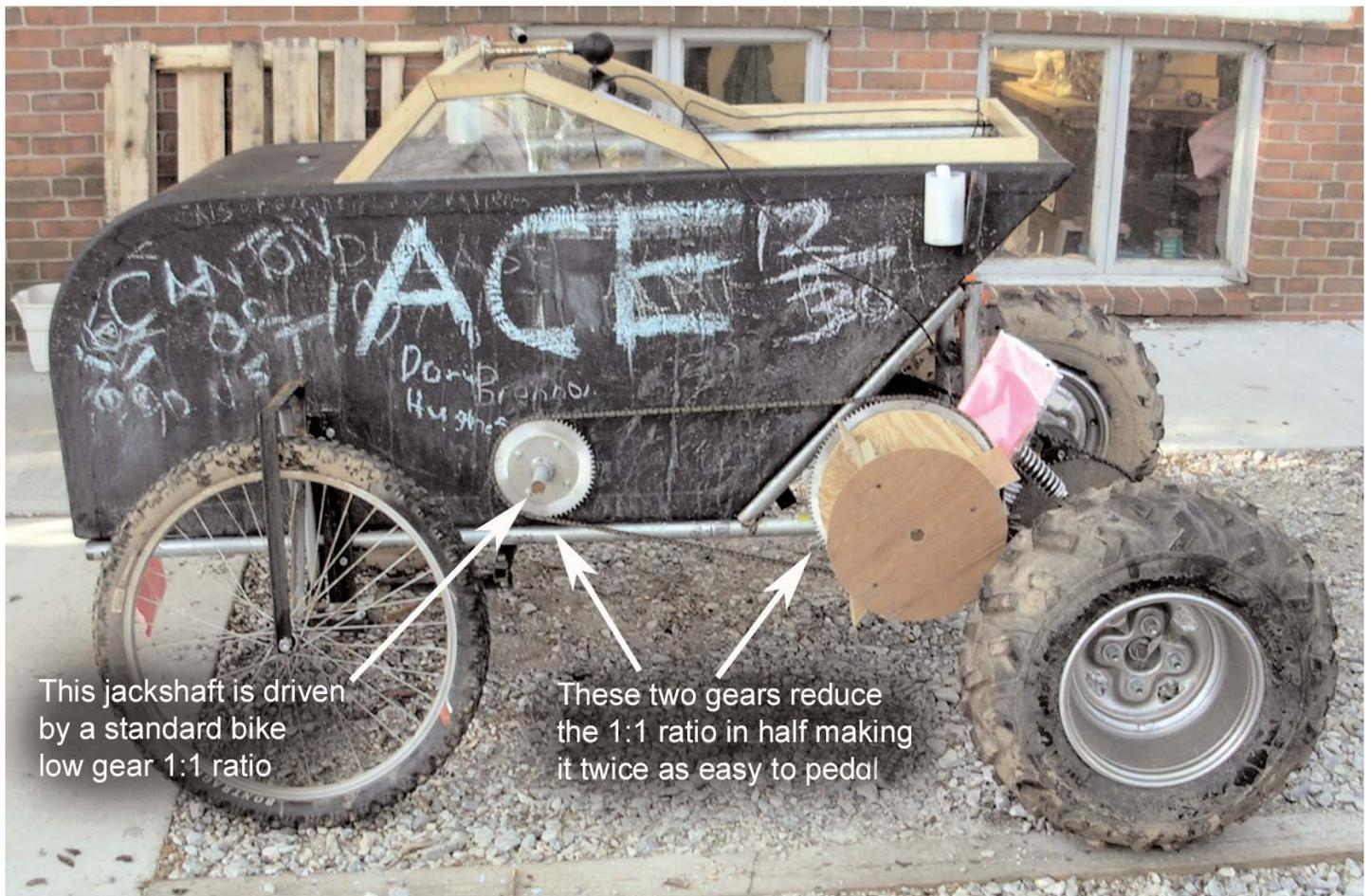
This jackshaft is driven by a standard bike low gear 1:1 ratio
