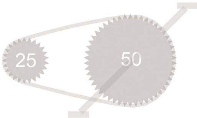
**HIGH GEAR**- A big gear in front and a small gear in back makes it *hard* to pedal and you go *fast*.
