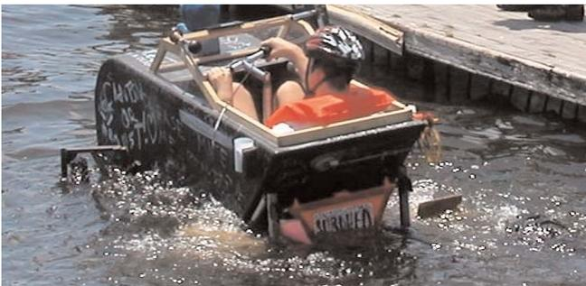
The vehicle on the left had simple paddle wheels mounted straight to a jackshaft already in the drive train. In both buoyancy calculations and water tests the expected waterline put about 1/3 of the paddle wheel submerged. Unfortunately some last minute alterations to the vehicle increased the weight in the rear. The actual waterline was higher and left the paddle wheels fully submerged and useless. The pilot prevailed and used an oar to successfully navigate the water.
